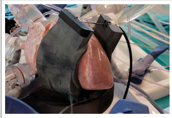
Figure 1. DCC patch device. The patches are in direct contact with the heart and are actuated through the driveline.
