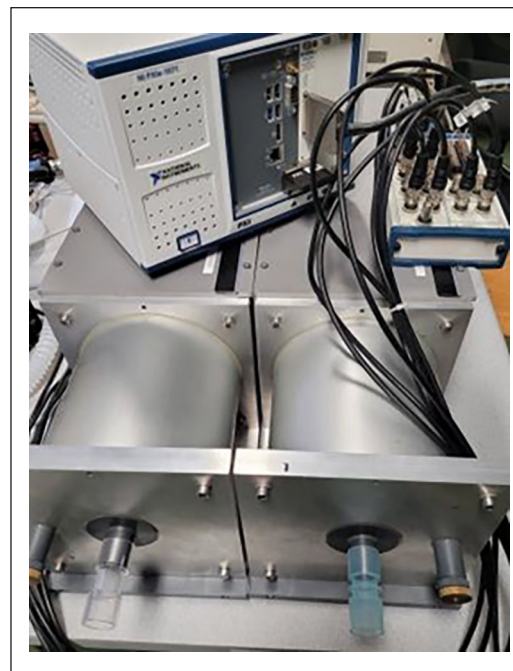
Figure 1. The hardware of the hybrid respiratory simulator, two piston-based pressure sources, and the computer simulating the pathophysiology of the respiratory system in real time.
